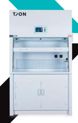
Ductless fume cupboards are the alternative to a fully ducted system. They take air from the room, pass the contaminated air through a filter(s), and release the clean air back into the room.
