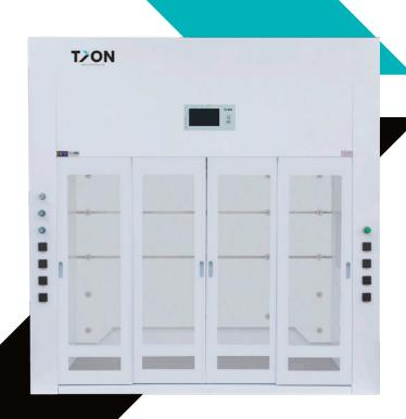
TION's walk-in fume cupboards safely house heavy or large equipment and materials that cannot be contained inside a regular fume cupboard. Helping to shield laboratory workers and protect sensitive processes.
